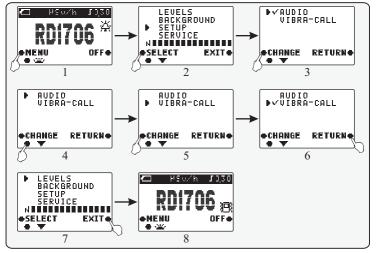
From this moment a vibra signal turns on if the value of a dose rate exceeds the installed threshold of alert when a threshold function is not turned off (page 15). A vibra signal starts functioning in a pulse-mode till the end of an observation cycle.
