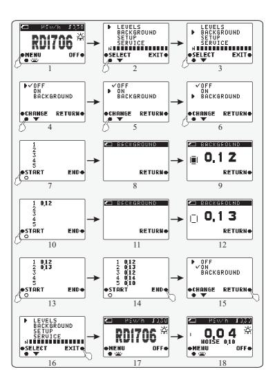
Press **«START»** button and wait till completion of the cycle of **«BACKGROUND»** estimation (screen 13). A value in the second line is the evaluation of a dose rate in the second sighting point (screen 14). In order to receive accurate estimation of a background it is necessary to conduct similar observations in 5 sighting points (screen 15).
