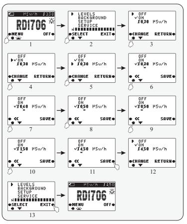
Press «**SELECT**» button and the screen 3 will appear. A double-click on «  $\blacktriangledown$  » button (screens 4 and 5) moves the cursor «  $\blacktriangleright$  » to «0,30  $\mu$ Sv/h».
